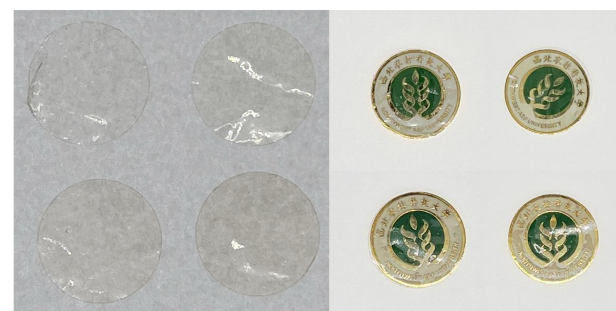
Fig. 1 Preparation of gelatin-TA composite films. The TA addition were 0, 0.5%, 1.0%, and 2.0 % of gelatin weight, respectively.
